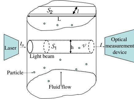
Fig. 1. Laser extinction measurement system
