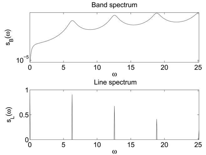
Fig. 5. Intensity power spectrum (first four harmonics) of an optical pulse train submitted to dependent jitter with Gaussian distribution of variance  $a^2$  and exponential correlation  $r_n = b^2 e^{-\nu|n|}$  ( $\Delta t = 10^{-3}$ ,  $T = 1$ ,  $a = 0.001$ ,  $b = 0.005$ ,  $\nu = 0.5$ ).
