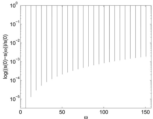
Fig. 1. Relative variations of the intensity power spectrum of a deterministic optical pulse train in logarithmic scale over the first 25 harmonics ( $\Delta t = 10^{-3}$  and  $T = 1$ )
