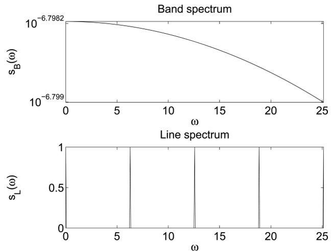
Fig. 7. The intensity power spectrum (first four harmonics) of an optical pulse train submitted to independent width modulation ( $\Delta t = 10^{-3}$ ,  $T = 1$ ,  $a = 0.001$ ,  $v = 0.001$ ).
