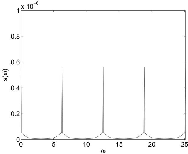
Fig. 3. Intensity power spectrum (first four harmonics) of an optical pulse train submitted to dependent amplitude modulation modeled by an autoregressive process with parameter  $[1 - 0.5]$  ( $\Delta t = 10^{-3}$ ,  $T = 1$ ,  $E[A]^2 = 0.5$ ).
