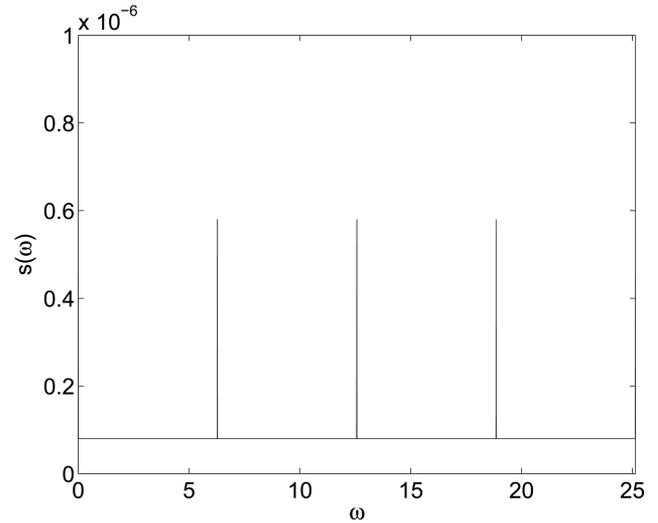
Fig. 2. Intensity power spectrum (first four harmonics) of an optical pulse train submitted to independent amplitude modulation with unit energy ( $\Delta t = 10^{-3}$ ,  $T = 1$ ,  $E[A^2] = 1$ ).
