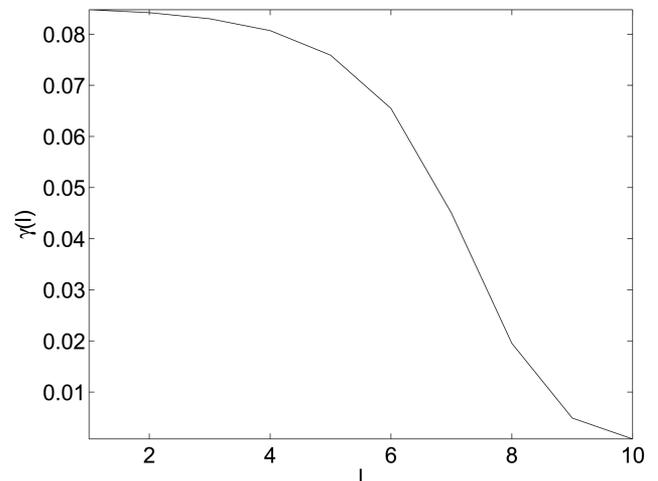
Fig. 6. Ratio between the consecutive line heights and the band spectrum (first 10 harmonics) in the case of dependent jitter ( $\Delta t = 10^{-3}$ ,  $T = 1$ ,  $a = 0.001$ ,  $b = 0.005$ ,  $\nu = 0.5$ ).
