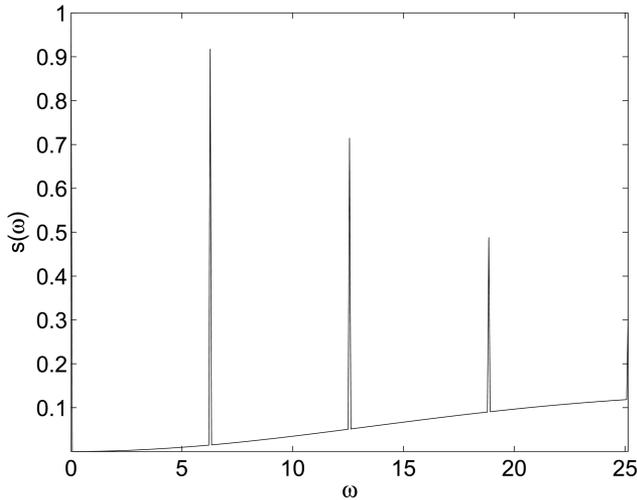
Fig. 4. Intensity power spectrum (first four harmonics) of an optical pulse train submitted to independent jitter of strength  $1/b$  and Gaussian distribution with variance  $a^2$  ( $\Delta t = 10^{-3}$ ,  $T = 1$ ,  $a = 0.01$ ,  $b = 0.05$ ).
