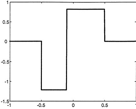
Fig. 11. Optimal wavelet for an AC embedded in white multiplicative noise ( $A = 0.5$ ).
