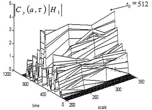
Fig. 9. CWT of a ramp ( $A = 0.4, t_0 = 512, a_0 = 200$ ) embedded in multiplicative noise with Haar wavelet.
