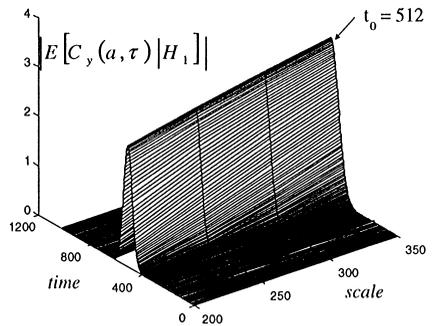
Fig. 3. Step signature ( $A = 0.4, t_0 = 512$ ) with FDG wavelet.
